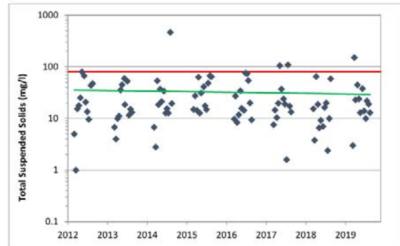
TSS sample results captured during annual monitoring at South Ecorse Creek site from 2012 to 2019. The red line indicates the 80 mg/L threshold. The green line indicates the trend.
